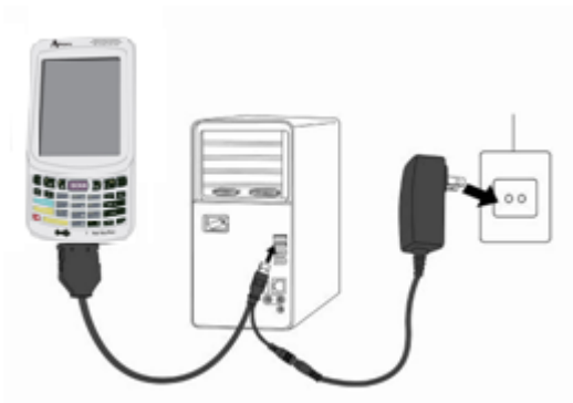
Figure 2-11 Communication through Cable
